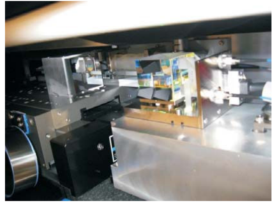
Fig. 7. Laboratory system: Aerotech stage and IF with multi-segment detector.
